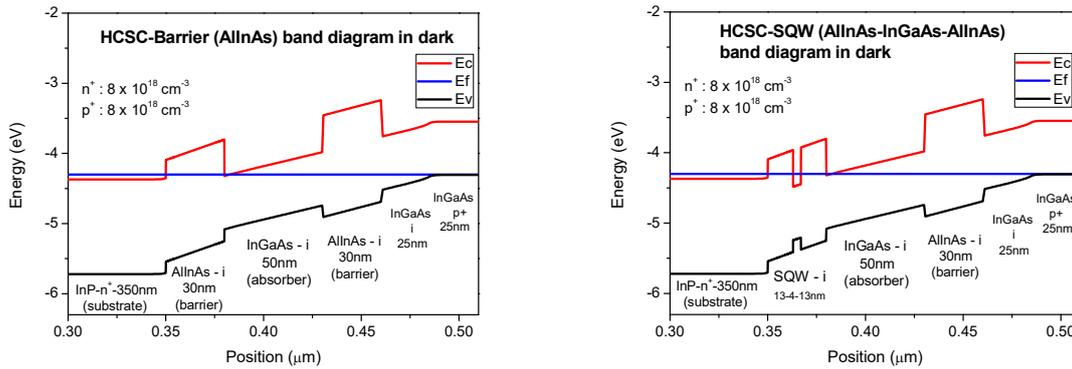
Fig. 1. Band diagram of HCSC barrier (left) and SQW (right) samples in dark
