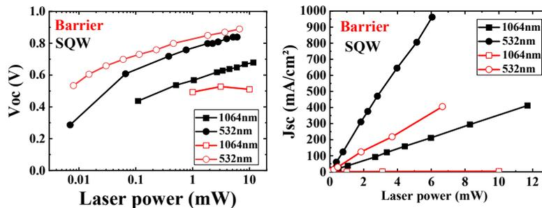
Fig. 2.  $V_{oc}$  (left) and  $J_{sc}$  (right) values as a function of laser power under different laser wavelengths for the Barrier sample (red) and for the SQW sample (black)
